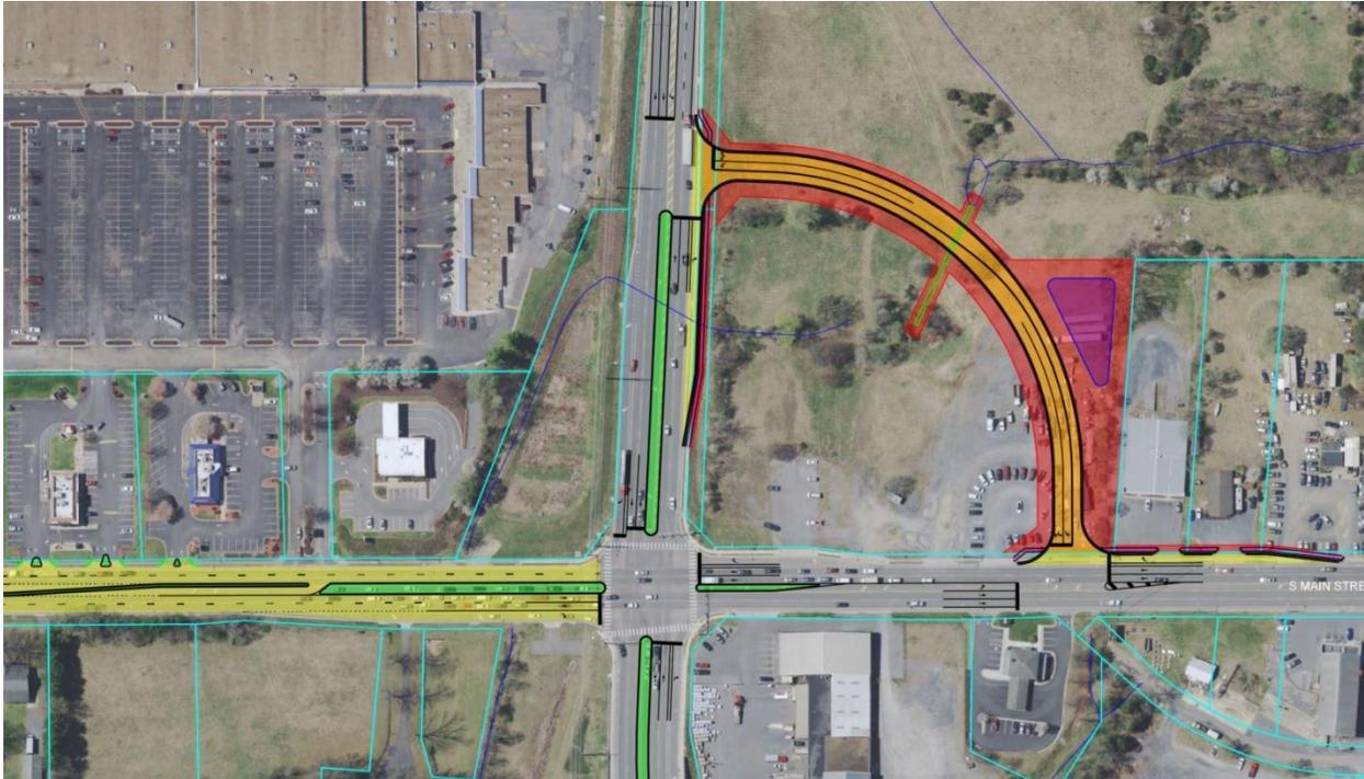
Figure 4: Alternative 2A Proposed Geometric Layout
