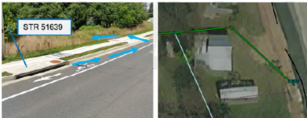
Figure 3: Structure 51639 Surcharge Routing
