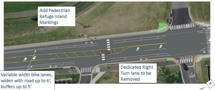
Garbers Church Road at BSES
