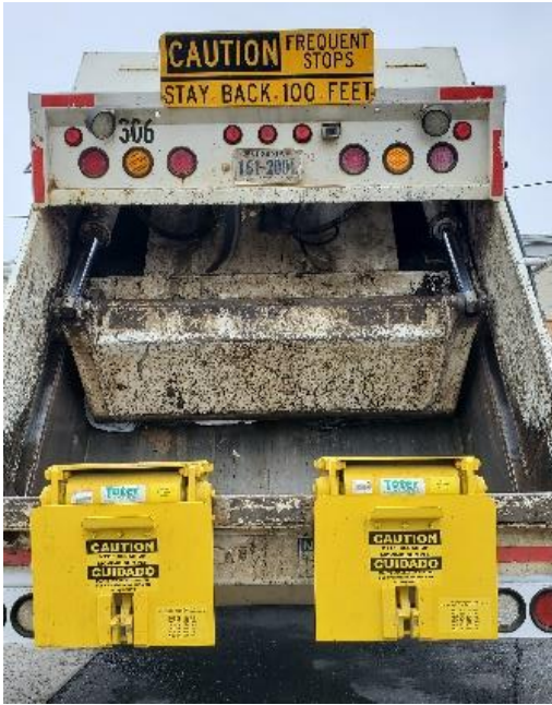
(Above) A truck retrofitted with tippers.
