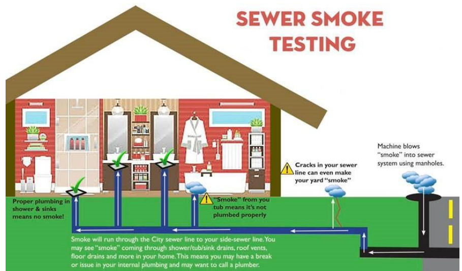
(Above) This graphic shows how the annual testing works, and where residents may notice some smoke. Testing begins on Monday, Sept. 9.
