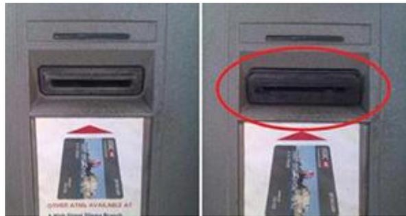
*This is not a photo from the station. It is a sample picture with a comparison of a card reader with a skimming device attached (red circle) and without a skimming device.*
