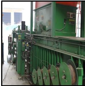
**20. Marathon 1475 Compactor -** Any residual material that remains in our system goes onto a residual belt that feeds into the compactor and trailer.
