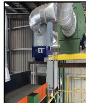
9. Main Sort Table - Where strategically placed drop chutes are placed over custom designed storage bunkers. Overhead the BloApCo suction system maximizes paper and plastic bag recovery. The strength of this process is the negative sort design. We are not using manual labor to do the work of machinery we are enhancing the recovery process by removing material that may have slipped through the cracks.
