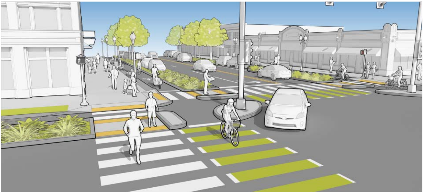
Figure 16: Design Elements of a Protected Intersection. Design elements include (1) a corner refuge island with a small curb radius, (2) a motorist yield zone, (3) bicycle queuing areas, and (4) marked pedestrian crossings.
