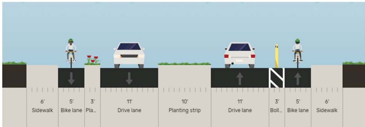
Figure 12: One-way Separated Bike Lanes Cross Section Example (Note: In most cases, the separation type would be the same on both sides of the street. This graphic shows a curbed planter strip on the left side and a paint-and-bollard design on the right side just to illustrate different options.)
